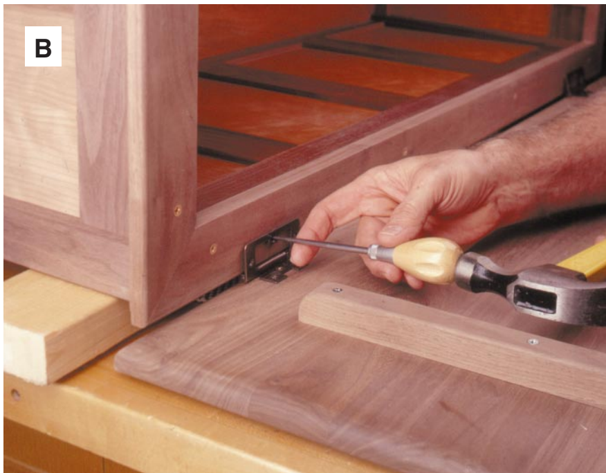
To locate the hinge positions on the back top trim (N), set the chest on 1½"-high support blocks (we used 2x4s). Position the top (P) as shown.
